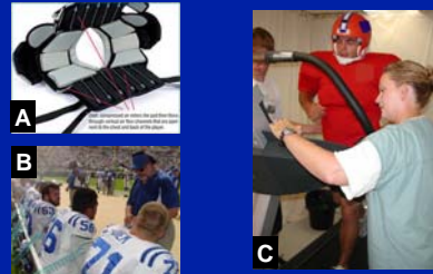
Figure 1. A. Shoulder pads with vertical air flow channels. B. Cooling system in use during a football game. C. Test subject running on the treadmill.
